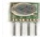
Figure 2. RF 434 Mhz Transmitter. Modulation: ASK
